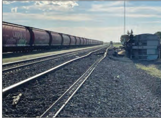
The north side of the main track looking west shows the second derailed car on its side. Further in the distance is the first derailed car which remained upright. | CANADIAN PACIFIC PHOTO
